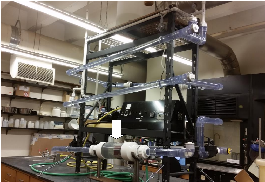
Figure 4.1 – Photograph of the continuous flow reactor system (28-Mar-16). A slurry of magnetic nanocomposite ion exchange (IX) particles is introduced to the wastewater stream at the top of the platform. Functional groups impregnated on the surfaces of the ion exchange particles bond with metal ions as the particle-laden stream is pumped through the reactor. The in-line electromagnet (see white arrow in the photograph) captures and retains the magnetic nanoparticles without impeding the wastewater flow. Periodically, the valve positions are changed to divert flow (through a parallel magnetic module) in order to strip the ions from the captured particles; after stripping, the electromagnet is de-energized to release the particles, which are filtered, reconditioned, and returned to service.
